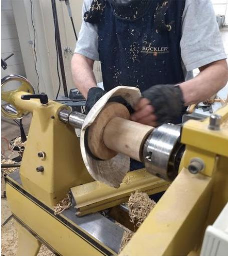
The final shaping of the foot of the finish-turned bowl is done using a jam chuck (left), with a mouse pad between the bowl and the jam chuck. Joe's setup included a removable extension cylinder between the jaws and the jam chuck, to accommodate bowls with tall sides.
