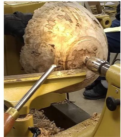
After: fully-rounded blank with tenon
