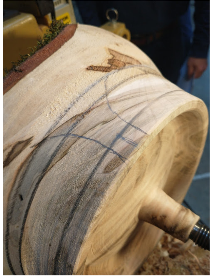
Right: The bottom of the bowl has been marked for the feet; the rest of it will be hollowed to a smooth curve transitioning from sidewall to rounded bottom.
