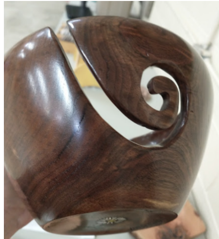
Robert Marshall showed a natural-edge bowl with severe tear-out, modified with thinned epoxy to permit a clean final cut. Left portion shows tear-out, right shows clean final cut. More info at our website.
