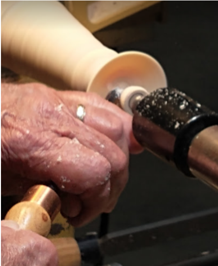
Left: carving the concave (top) side of the flower. Above: using lamp to gauge thickness, underside of flower.
