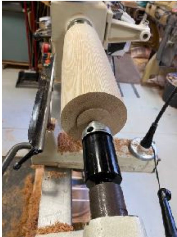
Blank is rounded with a tenon on each end
