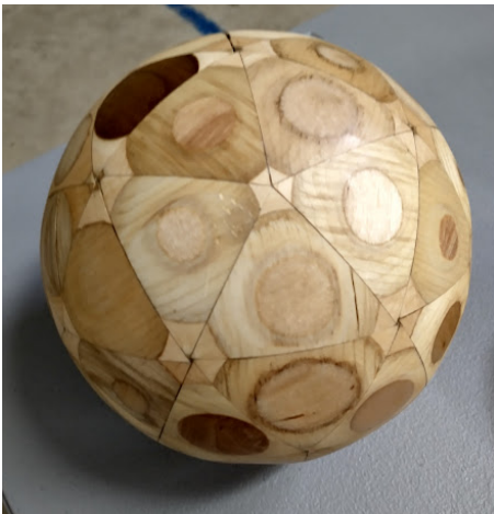
Robert Marshall turned this plywood sphere, assembled from 60 identical triangles, forming a 3-d geometric shape that was then turned on the lathe. More on website.
